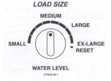
IMPORTANT: Holding the LOAD SIZE (WATER LEVEL) control in the RESET position can cause flooding of the washer.
