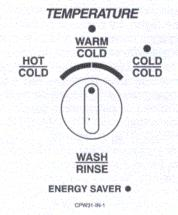
NOTE: The washer will provide a cold rinse in all TEMPERATURE settings. Cold rinses will save you money and energy and will help reduce wrinkling in permanent press and synthetics.
